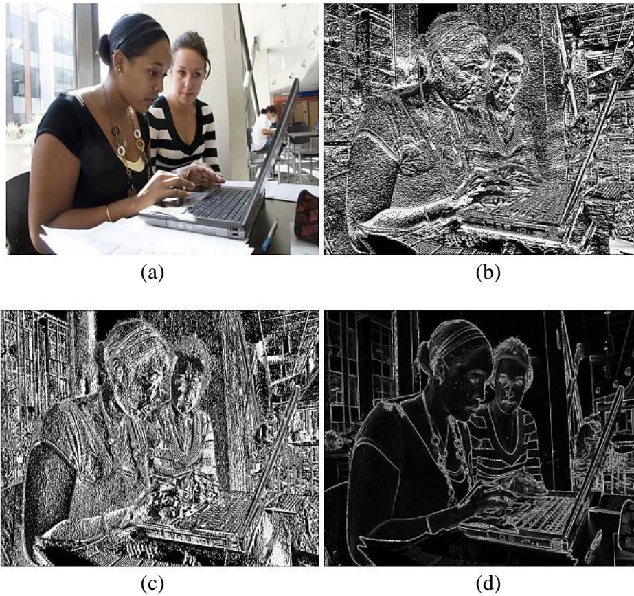
Figure 2.2: Spatial derivative of an image. (a) Original image, (b) partial derivative to x direction, (c) partial derivative to y direction and (d) spatial derivative of image.
