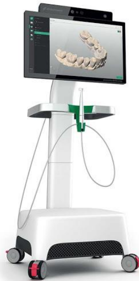
Fig. 5. The intraoral 3D scanner (The Straumann® CARES®, Craniofacial unit, Department of Oral and Maxillofacial Surgery, University of Szeged)
