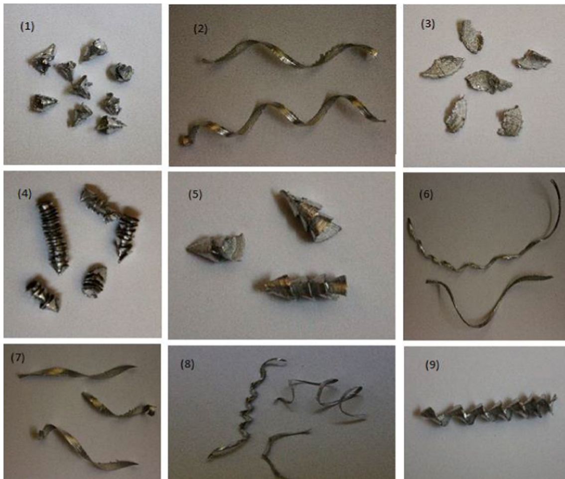
Fig. 6 Chips collected for each experiment on A6061T6
