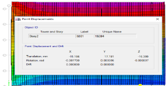
Fig.10. displacement at level C-south part of the building in Etabs T.D.P models for period 70 years
