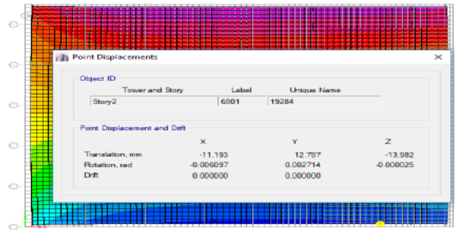
Fig. 9. displacement at level C-south part of the building in Etabs T.D.P models for period 4.5 years
