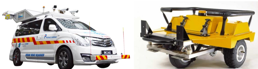
Figure 2. IKRAM Road Scanner (IRS) and Grip Tester (GT).
