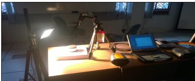
Figure 1. Solar reflectance measurement using Spectroradiometer.
