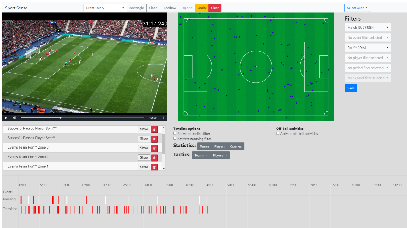
Figure 2: SportSense UI with video, drawing area, filter area, timeline, buttons for the statistical analysis, and dropdown menus for the tactical analysis. The visualized results show the Pressing Phases and offensive Transition Phases (of one team) of the first 45 minutes of the match.
