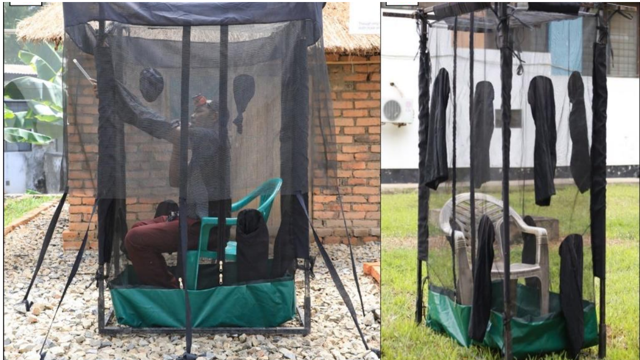
Figure 5.2. Photo of the miniaturized double net trap used to catch host-seeking mosquitoes. The miniaturized double net trap consists of an inner chamber, normally occupied by adult volunteer mosquito catchers. There is an outer netting cover, hanging 80cm from the ground, which traps host-seeking mosquitoes attempting to reach the volunteer inside. Host-seeking mosquitoes are trapped between the inner and outer netting compartments and are collected by the volunteer through the multiple sleeves which open outwards from the inner compartment using a mouth aspirator.
