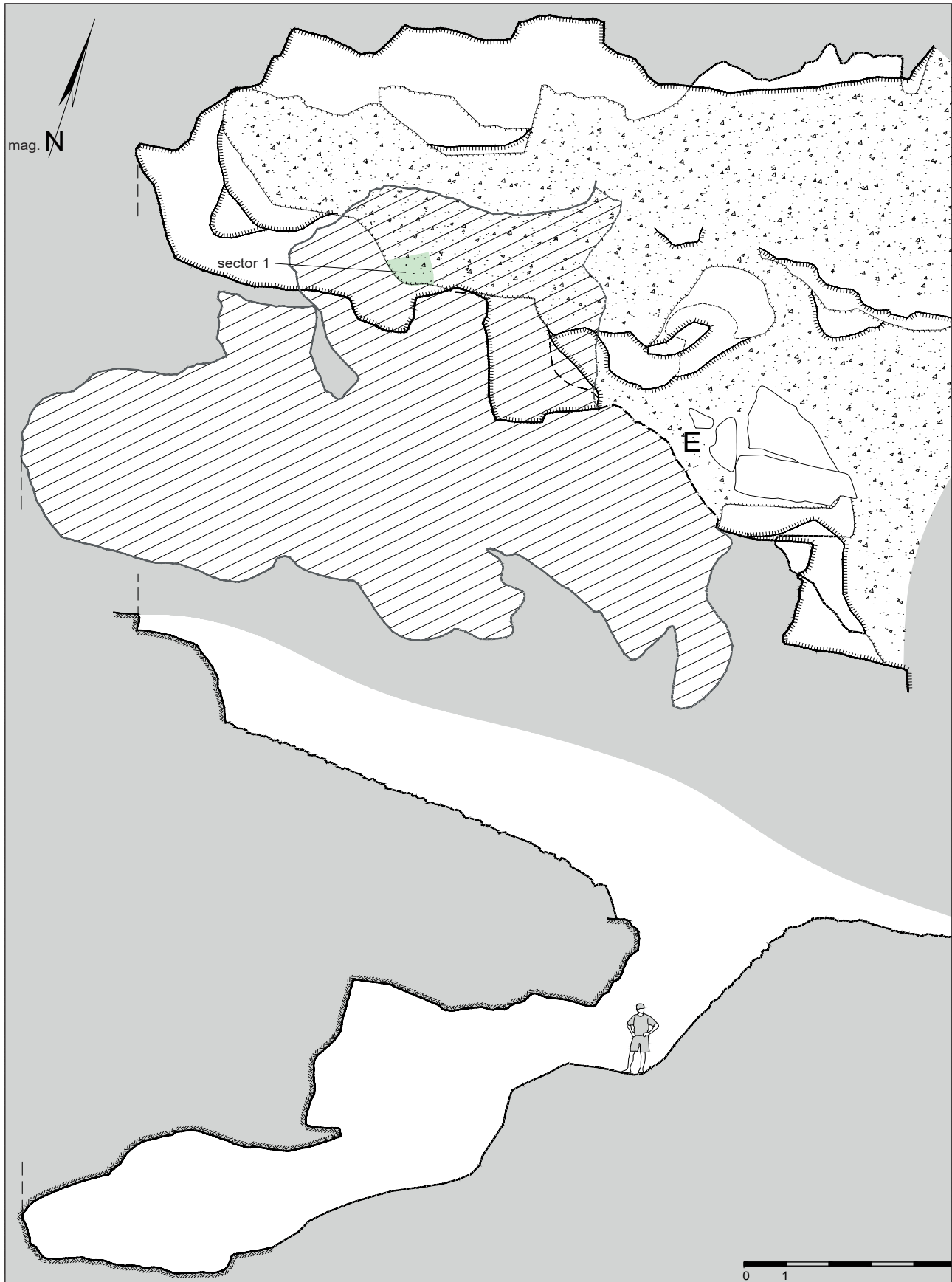
Fig. 13. Cotschens, mine 1, opencast with underground cavity. – Top: ground plan. – Bottom: vertical projection (Plan: P. Thomas and G. Steffens, DBM).
