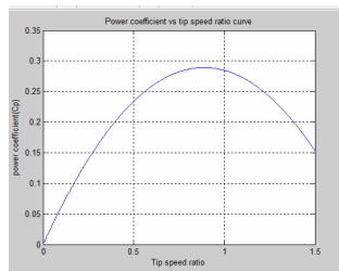
Figure 6.5: Power coefficient versus tip speed ratio curve
