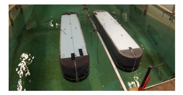
Figure 3.1: Ship Models in Waves
