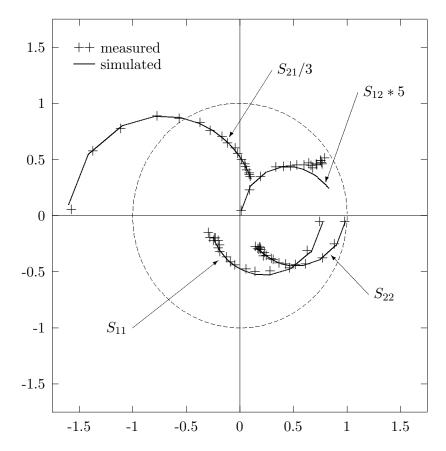
Fig.7. HBT S-parameters as functions of frequency; extracted values of parameters.
