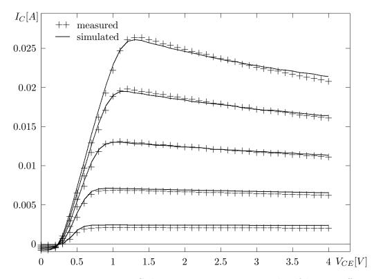
Fig.10. HBT common–emitter DC characteristics; extraction with self–heating effects.
