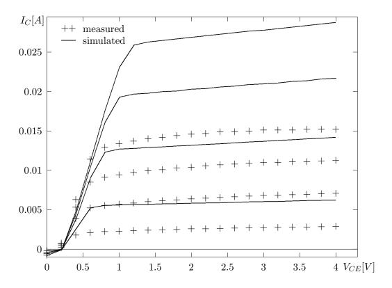
Fig.4. HBT common–emitter DC characteristics; initial values of parameters.
