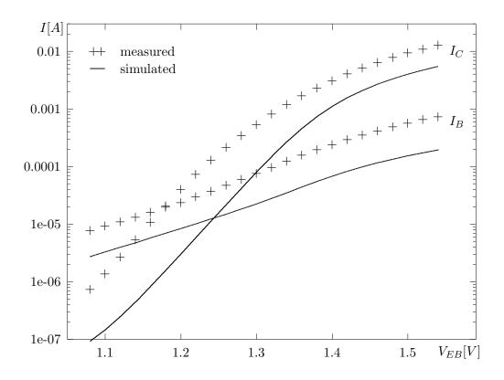
Fig.2. HBT common–base DC characteristics; initial values of parameters.
