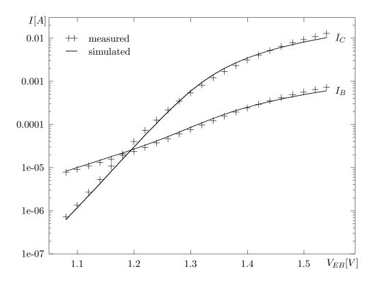
Fig.3. HBT common–base DC characteristics; extracted values of parameters.
