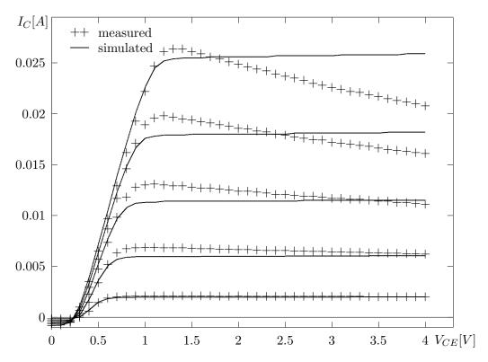
Fig.9. HBT common-emitter DC characteristics; extraction without self-heating effects.
