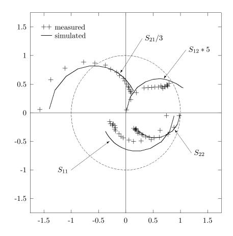
Fig.6. HBT S-parameters as functions of frequency; initial values of parameters.
