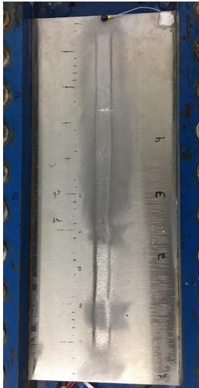
Figure 7.2:59 – Crack at 265 Vpp for a sweep test with all piezoelectric actuators activated in phase from 1985 Hz to 2035 Hz in 10 seconds
