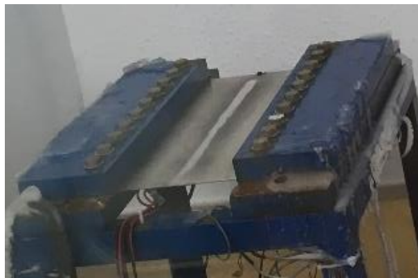
Figure 7.1:12 – Final state of the ice layer after steady-state tests at 188 Hz, 185 Hz and 183 Hz
