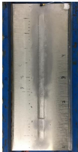
Figure 7.1:15 - Cracking of the ice layer in steady-state mode at 1338 Hz and 320 Vpp
