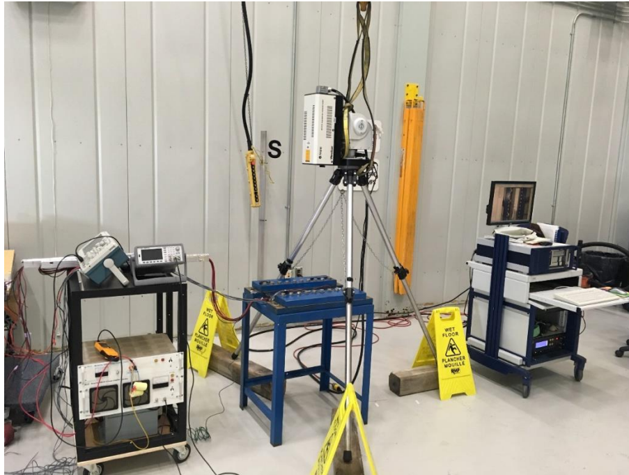
Figure 4.3:1 – Flat plate setup at NRC Ottawa for laser vibrometer measurements
