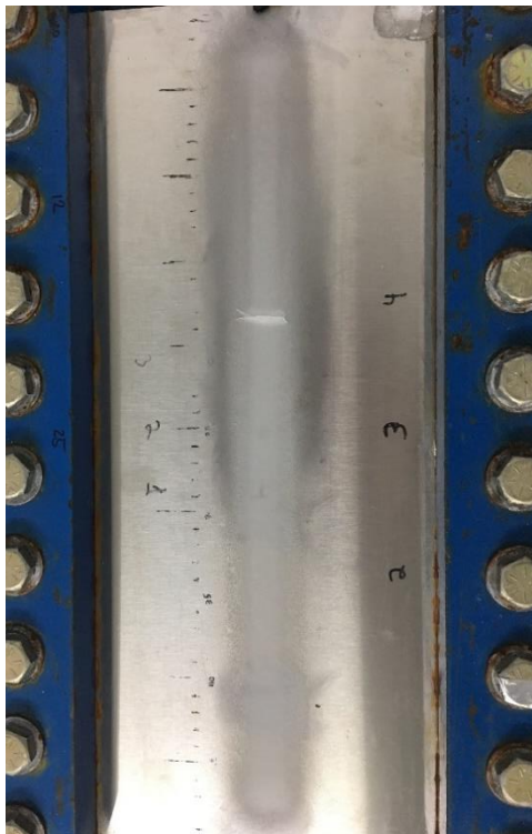
Figure 7.2:49 – Crack at 335 Vpp for a sweep test with all piezoelectric actuators activated in phase from 1575 Hz to 1625 Hz in 10 seconds
