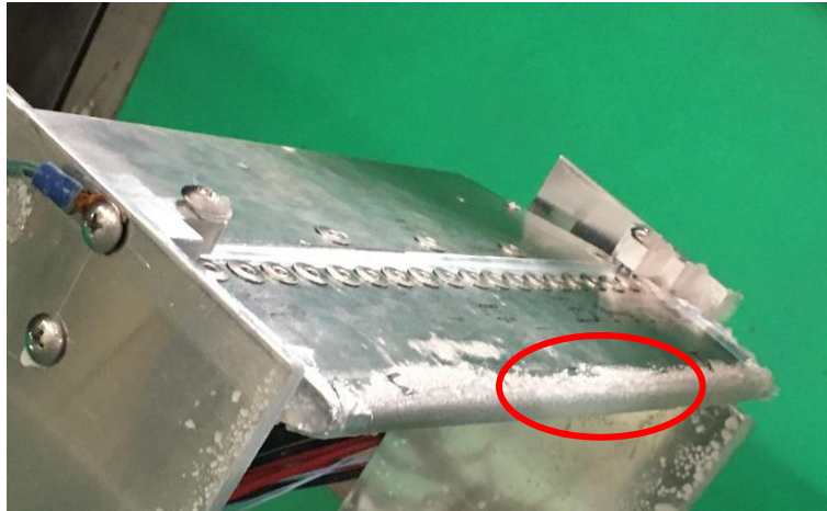
Figure 8.2:10 – Delamination of the ice layer for mode 5 during first repetition
