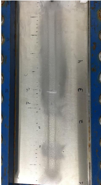
Figure 7.2:53 - Crack at 170 Vpp for a sweep test with piezoelectric actuator 3 out of phase with the 4 other piezoelectric actuators from 1575 Hz to 1625 Hz in 10 seconds
