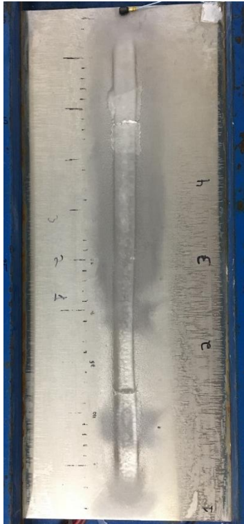
Figure 7.2:24 – Crack obtained after a sweep from 1300 to 1350 Hz in 10 s with all piezoelectric actuators activated in phase performed at 400 Vpp without any other sweeps performed before
