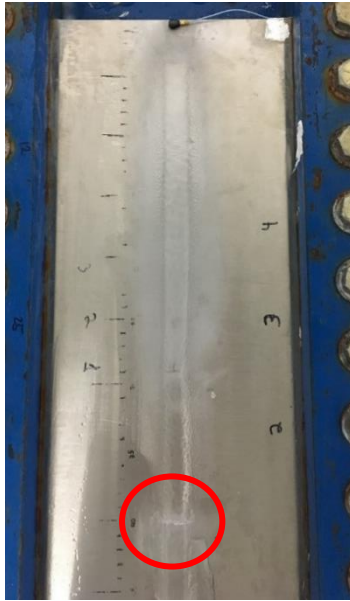
Figure 7.2:7 - Crack at 300 Vpp for a sweep test with all piezoelectric actuators activated in phase from 375 Hz to 425 Hz in 10 seconds
