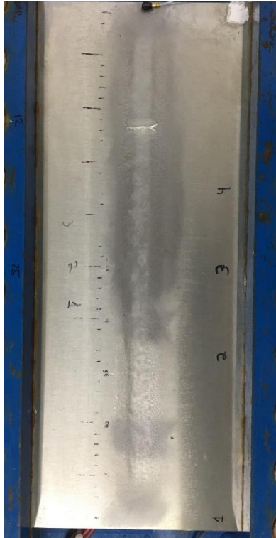
Figure 7.2:13 – Crack obtained after a sweep from 375 to 425 Hz in 10 s with all piezoelectric actuators activated in phase performed at 370 Vpp without any other sweeps performed
