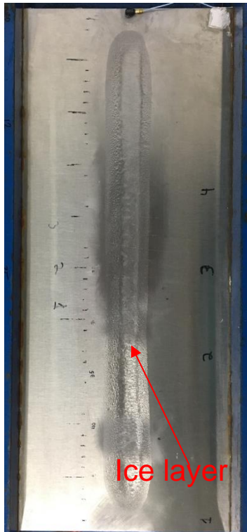
Figure 7.1:3 – Ice layer accumulated on the flat plate setup
