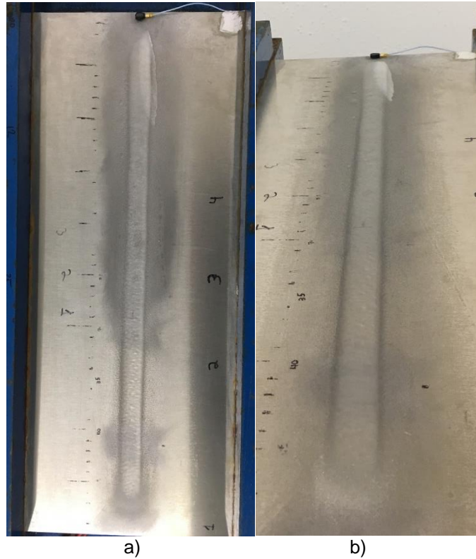
Figure 7.2:63 – Delamination at 216 Vpp for a sweep test with piezoelectric actuators 1 and 2 activated out of phase with 4 and 5 from 1575 Hz to 1625 Hz in 10 seconds a) top view b) side view
