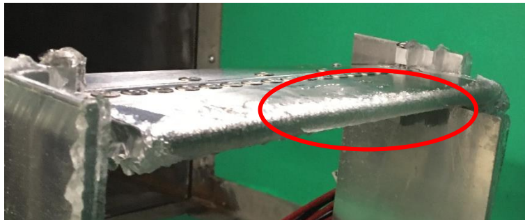
Figure 8.2:12 – Delamination at 352 Vpp for mode 5 repetition 2 with all piezoelectric actuators excited in phase
