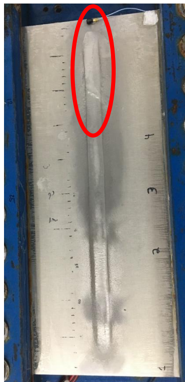
Figure 7.2:33 – Delamination at 192 Vpp for a sweep test with all piezoelectric actuators activated in phase from 1130 Hz to 1180 Hz in 10 seconds
