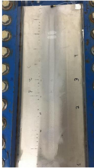
Figure 7.2:15 - Crack at 216 \text{ Vpp} for a sweep test with piezoelectric actuators 2 and 4 out of phase with the 3 other piezoelectric actuators from 375 \text{ Hz} to 425 \text{ Hz} in 10 seconds
