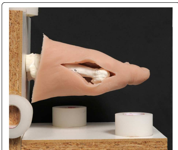
Fig. 1 Foot dummy. The approach through the silicon reveals the exchangeable polyamide MT I
