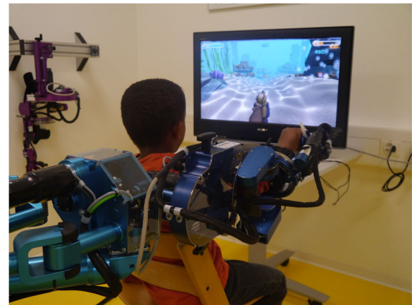
Fig. 2 The ChARMin robot. The ChARMin exoskeleton: a young boy practicing with ChARMin’s small distal module
