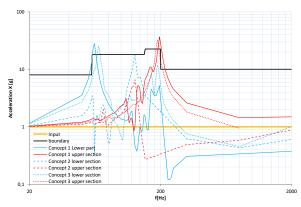
Figure 19: dynamic response in axial direction (X). All results are normalized to an input of 1g
