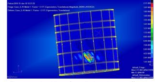
Figure 14: buckling of a cylinder with 16 stiffeners, one additional frame and a skin thickness of 1.0mm
