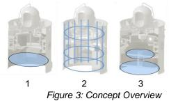
The main difference of the concepts is the accommodation of the units. The position of the aerodynamic fins and the reaction system is the same for all concepts. This includes that the inertia box as support of the fins is geometrically similar across the concepts. The structural material is set to be aluminium.
