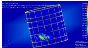
Figure 15: buckling of a cylinder with 16 stiffeners, one additional frame and a skin thickness of 1.2mm
