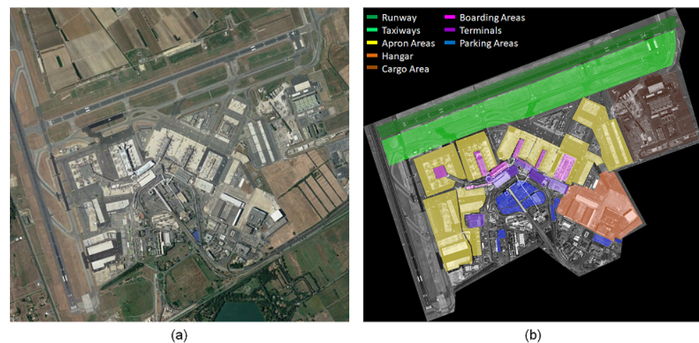
Figure 1. Rome–Fiumicino International Airport: (a) Google Earth view of the analyzed area and (b) geocoded masks superimposed to Pleiades image.
