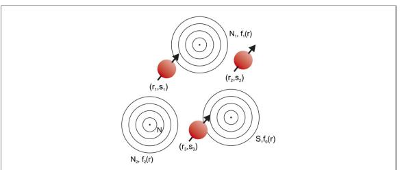
**Figure 1.** A network of quantum sensors described by their locations  $r_j$  and internal spin  $s_j$  can distinguish between the signal S and different noise sources  $N_k$  due to their different spatial distributions  $f_k(r)$ .
