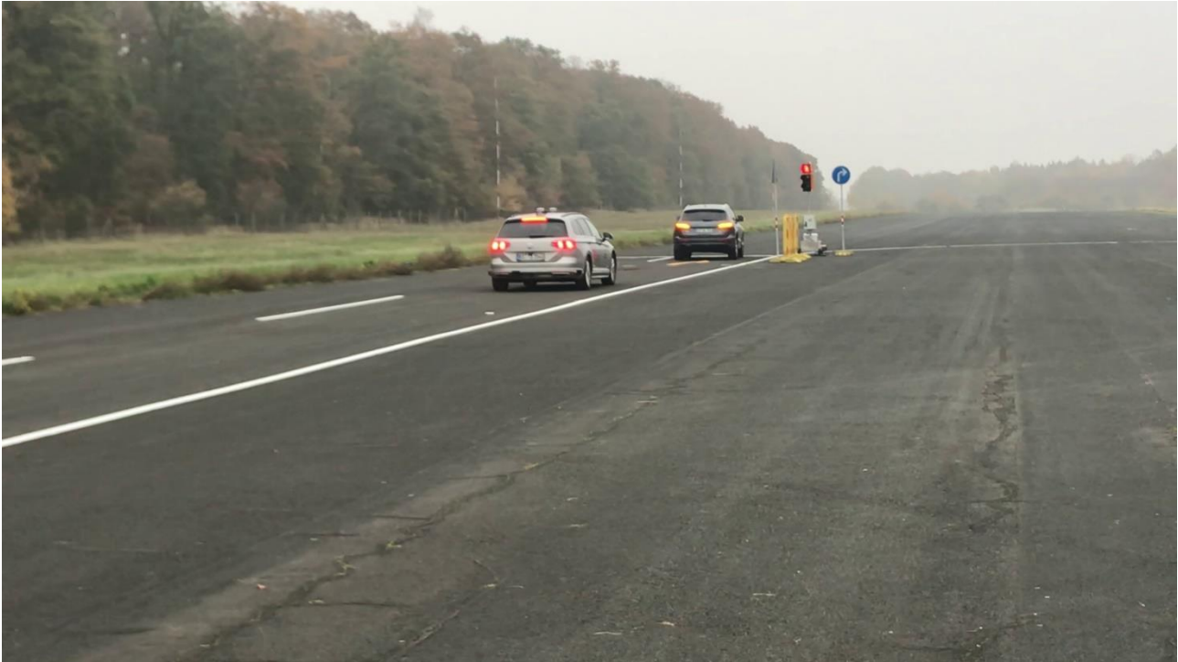
Figure 48: ViewCar2 stopping behind broken-down vehicle.
