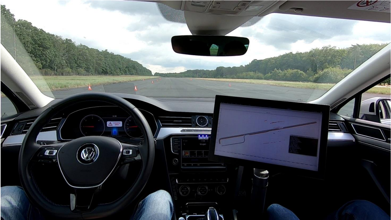
Figure 24: Execution of the MRM inside the ViewCar2. Blockage indicated in digital map by DENM reception at the position of the cones on the road, left side.
