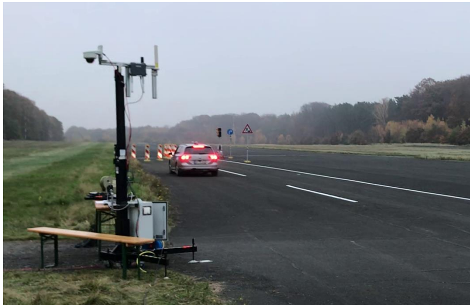
Figure 55: ViewCar2 performing the MRM in the safe spot on the left lane.
