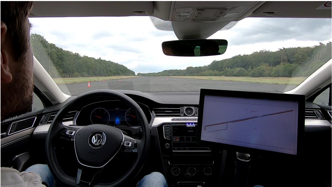
Figure 25: ViewCar2 executing the lane change around the blockage.
