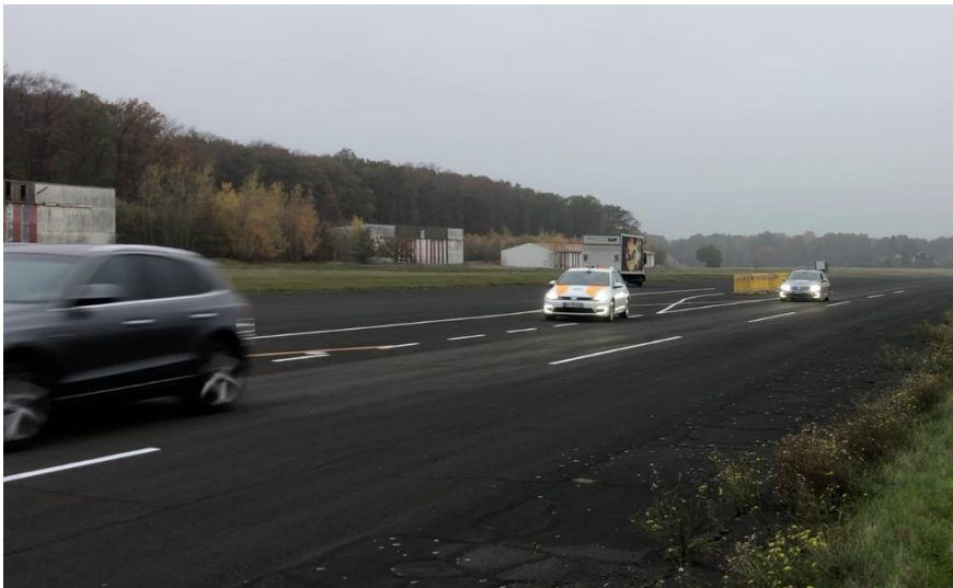
Figure 45: The CAV on the highway opens a gap for the merging vehicle by using V2V communication
