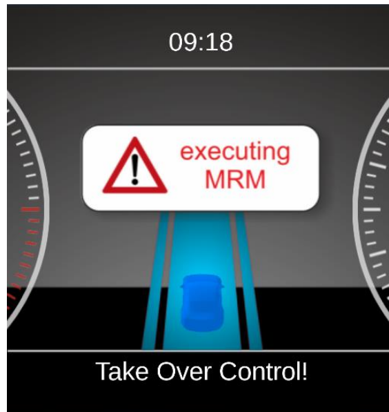
Figure 12: HMI showing active Minimum Risk Manoeuvre
