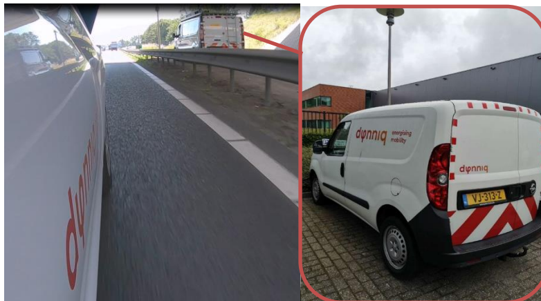
Figure 62: A service van facilitated to a mobile RSU station
