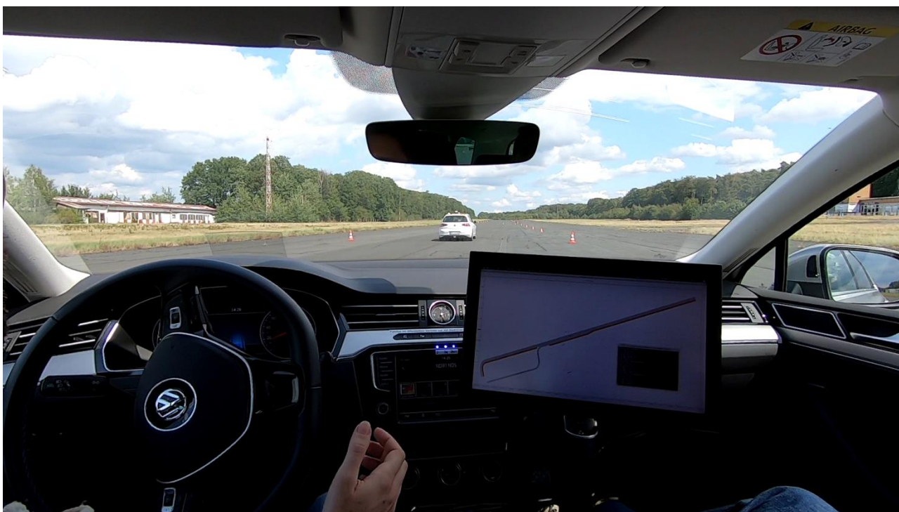
Figure 30: Successful lane change after speed adaptation of ViewCar2 on the ramp.
