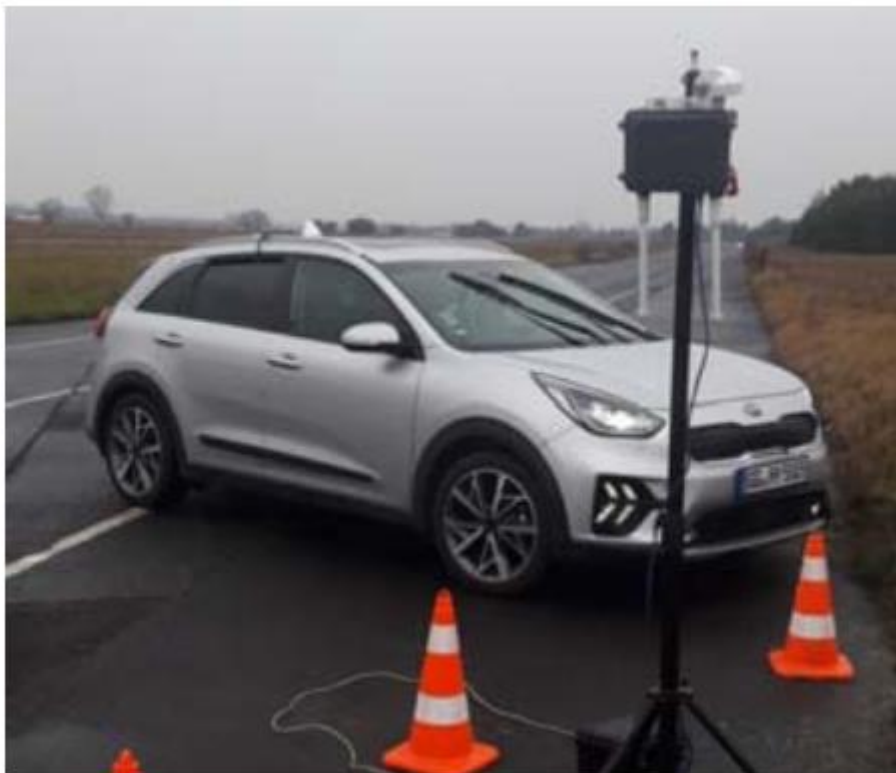
Figure 69: CAV and RSI prototypes
