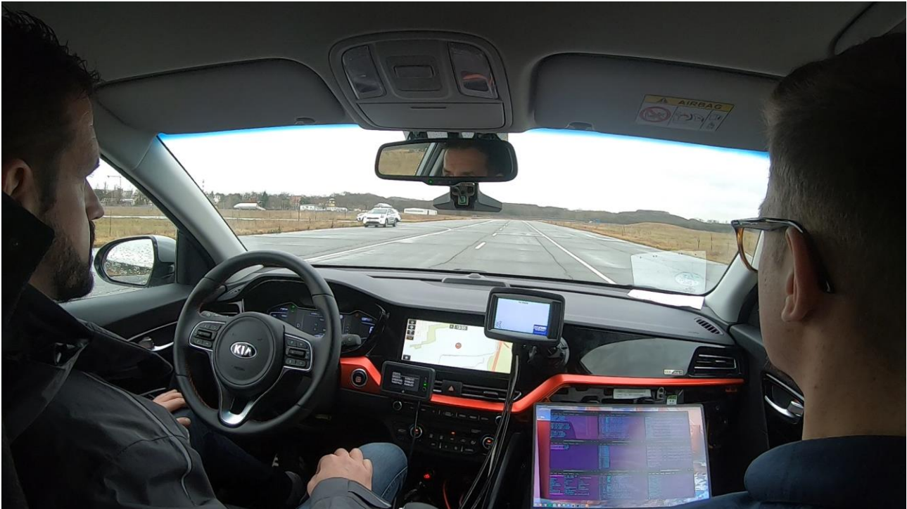
Figure 73: Execution of a parking manoeuvre at a safe stop on the emergency lane in reaction to an MCM reception
