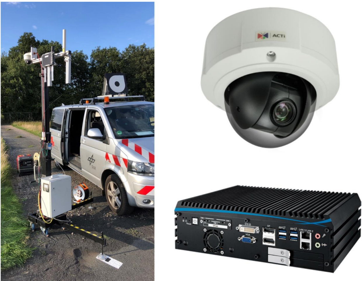
Figure 21: Mobile RSU with mounted ACTi Camera and ECX 1200 processing computer
