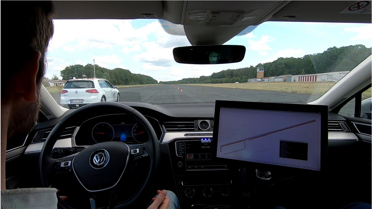
Figure 27: Blocked entrance, as manually driven FASCarE on adjacent lane does not allow merging (driving at the same speed). Lane change not possible, ViewCar2 stops.
