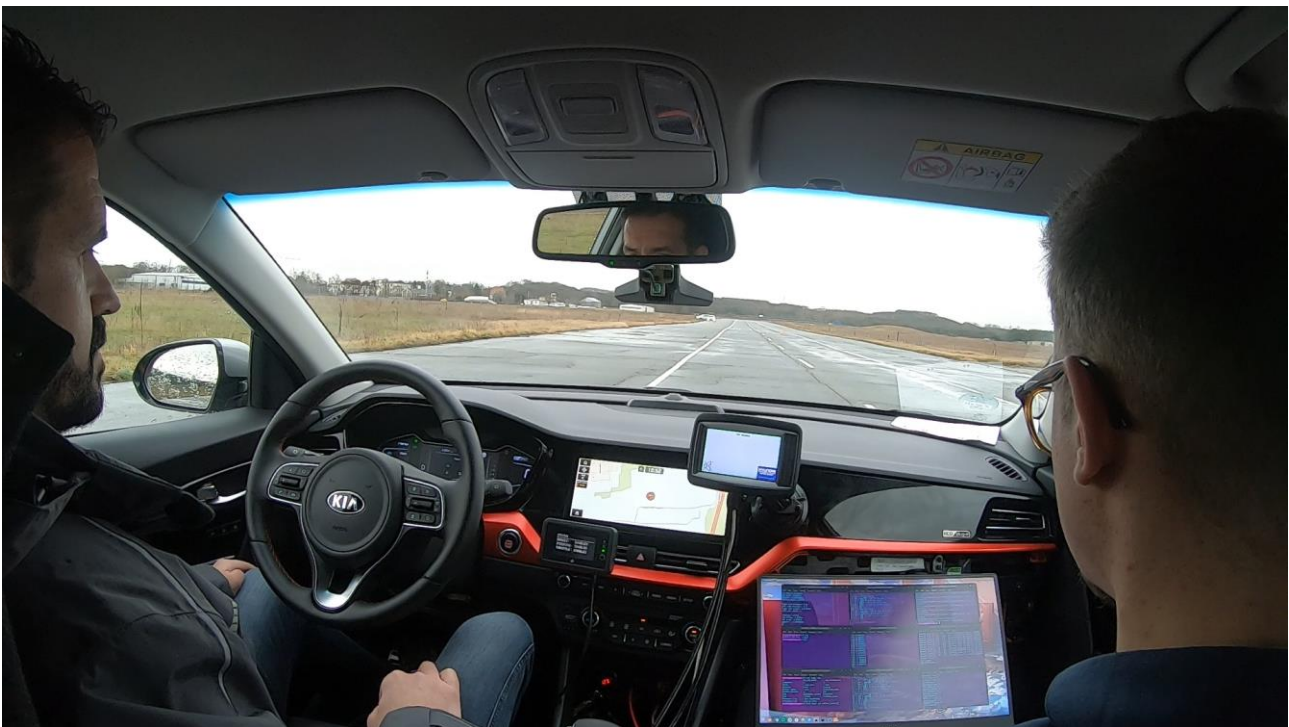
Figure 72: Execution of a parking manoeuvre on the driven lane in reaction to a DENM reception when no safe spot is available
