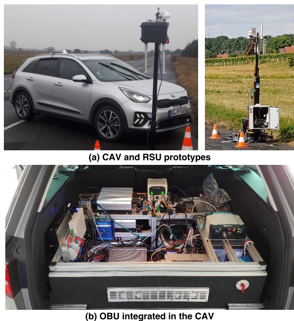
FIGURE 5. Prototypes used to collect V2X messages.
