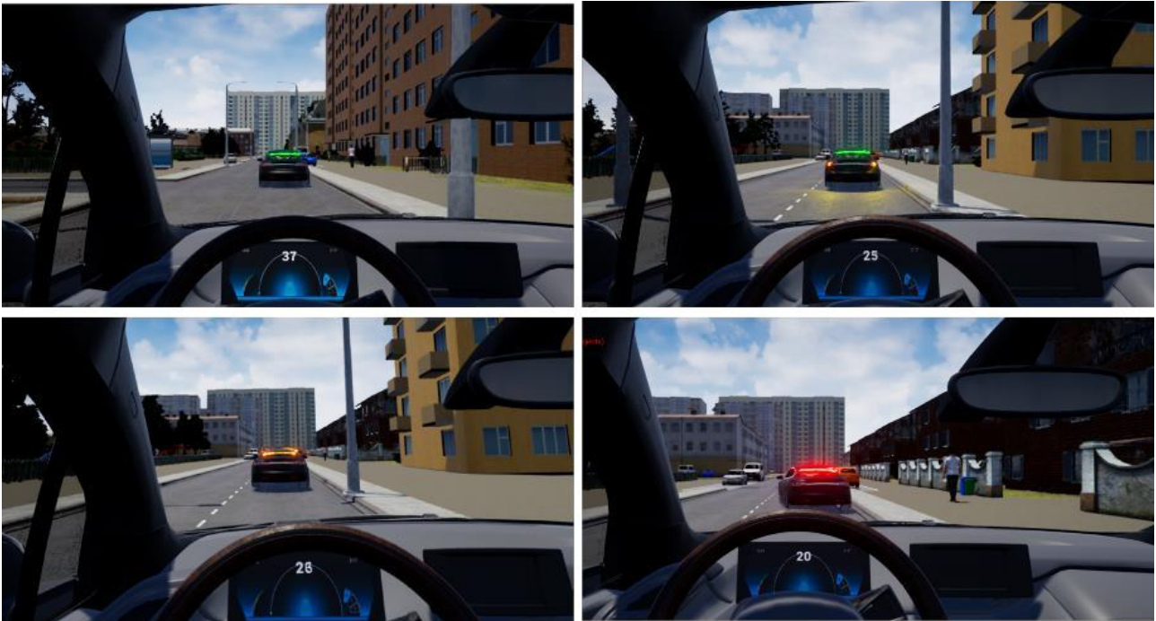
Figure 3: simulated external light strips to provide detailed information about the automation state and its goals
