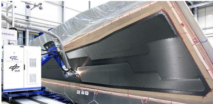
Large-scale components in Fiber-Placement-Technology (multi-robot-approach)
