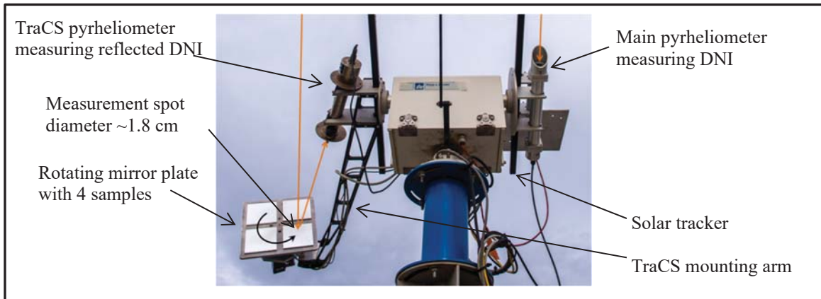
FIGURE 1. Updated TraCS4 measurement system at Plataforma Solar de Almería (PSA, Spain).
