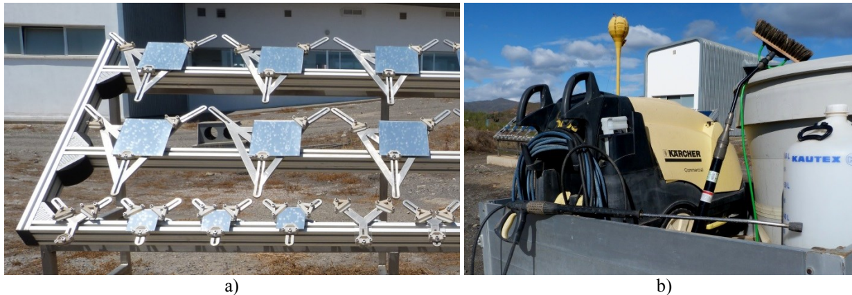
FIGURE 1. a) Outdoor exposure rack 1 with exposed samples, b) Kärcher cleaning device.
