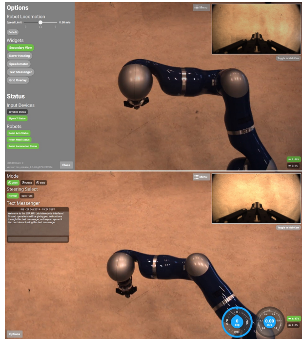
Fig. 4: The Astronaut GUI. Above: with the hideable sidebar, the astronaut can set the rover speed limit and select and deselect widgets. They can also see which input devices and robots are connected. In the image, only the secondary view is selected, and only the Joystick controls station is offline. Below: the view during messenger operation. The chat, speedometer, and bearing widgets are enabled.
