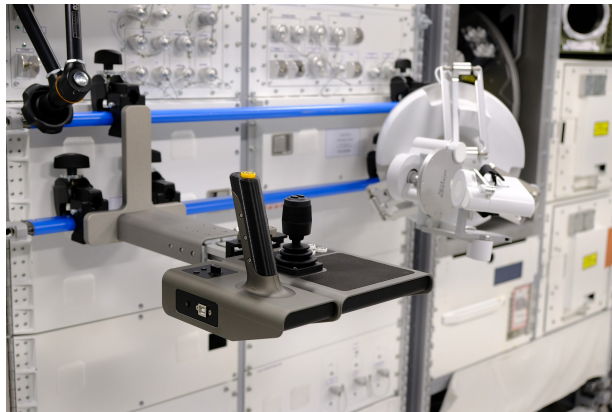
Fig. 3: Mounting of sigma.7 and joystick control station on the ISS. The laptop is above them, out of the picture.
