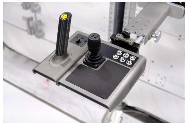
Fig. 2: Custom joystick control station with stabilisation handle and enable button (left), 3-axis joystick, and buttons.
