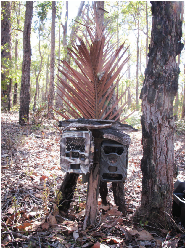
Fig. 2. Paired, side-by-side camera trap set up of periodically repositioned Reconyx (PC900, left), and Swift 3C wide-angle camera traps for the detection of wildlife in the Upper Warren region, Western Australia. Branches and leaves were used to conceal and disrupt the shape outline of camera traps and attachment structures.
