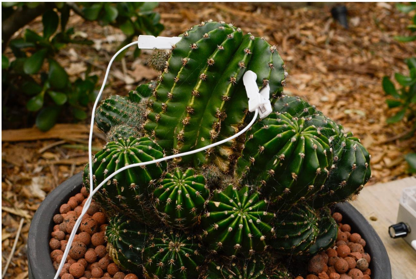
Fig. 4. A bio-sonification module attached to a cactus using ear clips for a TENS machine.
