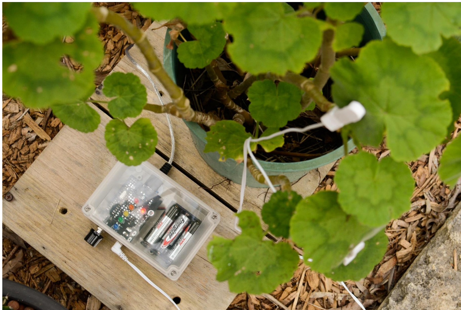
Fig. 3. A bio-sonification module attached to a geranium plant using ear clips for a TENS machine.
