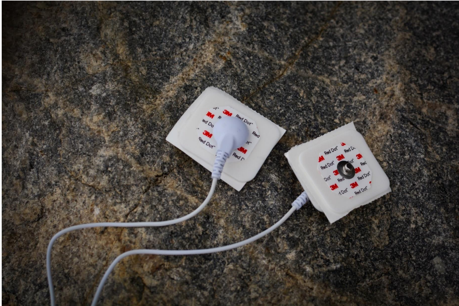
Fig. 5. Adhesive pads that are commonly used to transmit plants' electrical signals to a bio-sonification module.
