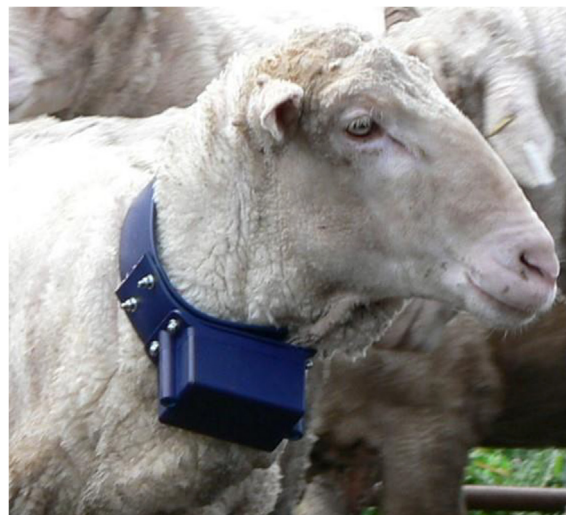
Fig. 2 – The GPS devices used to track sheep behaviour.
