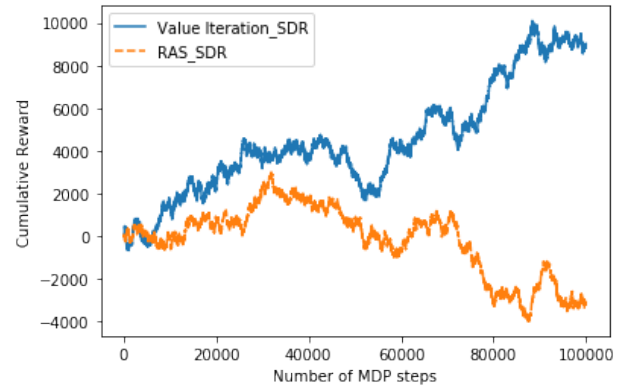
Fig. 5. Cumulative reward comparison between value iteration approach and RAS approach for an SDR MDP case
