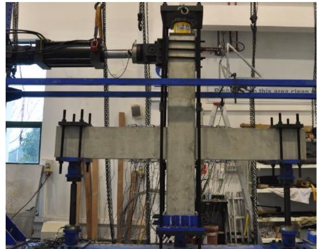
Figure 4. Test setup of BCJ specimens (Unit: mm).
