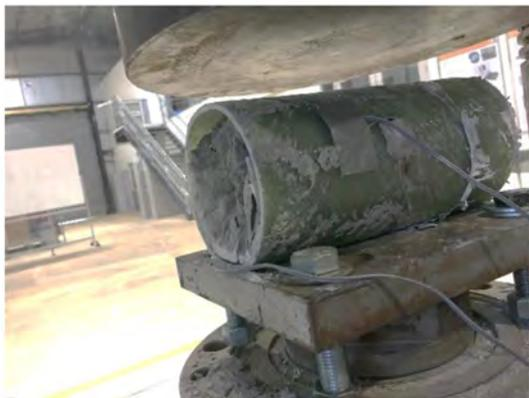
Fig. 2. Splitting tensile test set-up.
