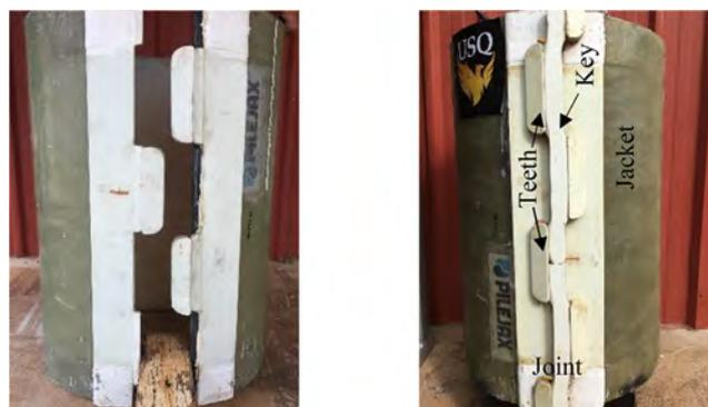
Fig. 1. Novel GFRP jacket with novel joining system.
