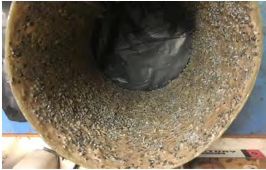
Fig. 4. Roughened GFRP tube.
