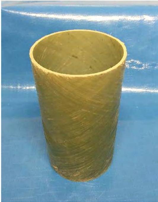
Fig. 1. The pre-fabricated GFRP tube.
