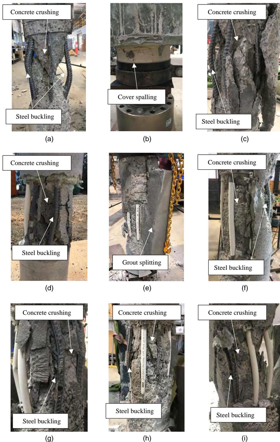
**Fig. 7.** Failure modes of tested columns: (a) C-0-0; (b) C-0-0-S; (c) C-0-0-J; (d) C-50-100; (e) C-50-100-G; (f) C-50-50-J; (g) C-50-100-J; (h) C-50-100-J\*; and (i) S-50-50-J.
