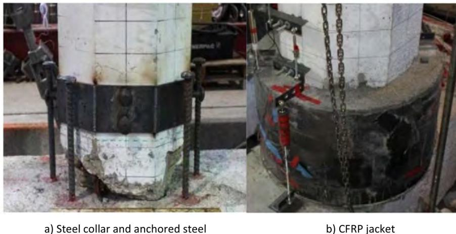
Fig. 8. Seismic repair method [26].
