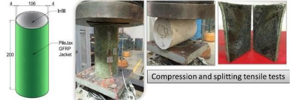
Compression and splitting tensile tests
