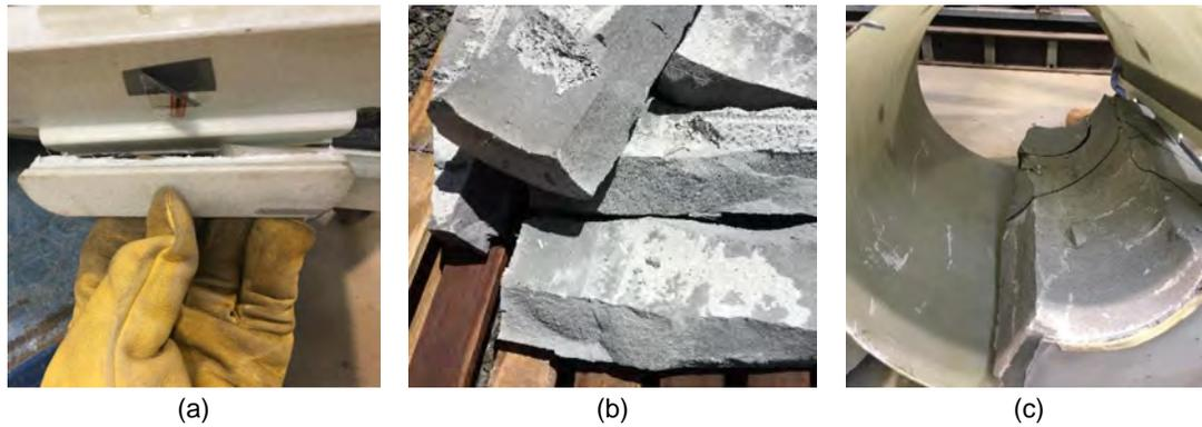
**Fig. 8.** Specific failures in components of repair system: (a) rupture of the GFRP jacket's teeth; (b) large pieces of broken grout infill; and (c) debonded GFRP jacket and grout infill.
