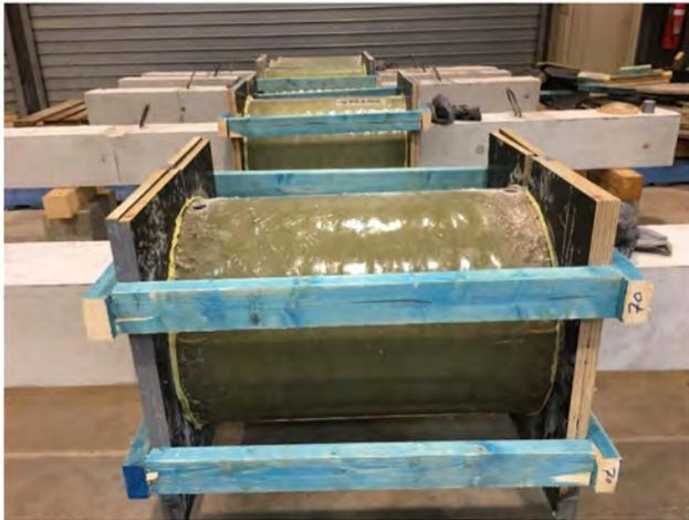
Fig. 7. Installation of GFRP jackets over the beams.
