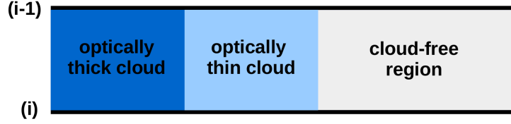
Figure 3.10: A model layer between levels (i - 1) and (i) divided into three regions.
