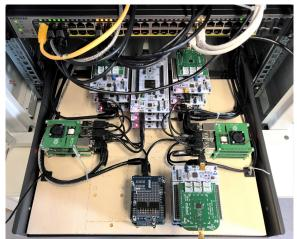
(b) All Nodes of the Testbed including the switch are assembled in a rack.
