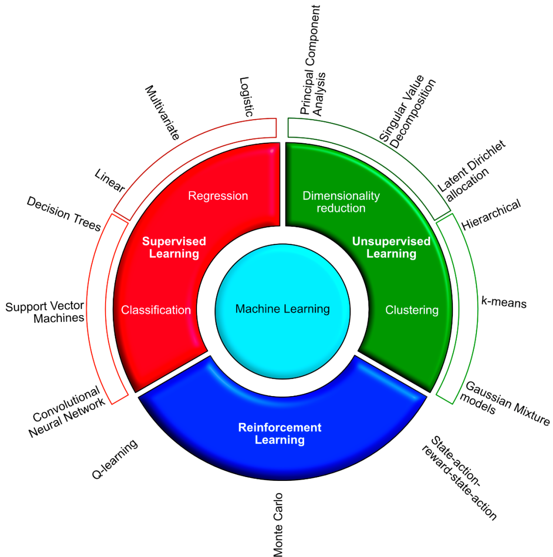
Figure 5. The three main types of machine learning approaches. Supervised machine learning algorithms are divided in classification and regression. Classification algorithms output a limited set of values (such as categorical or binary values), while regression outputs numerical values within a range. Examples for classification include Decision Trees, Support Vector Machines (SVM) and Convolutional Neural Networks (CNN). The most common regression algorithms include Linear, Logistic and Multivariate Regression (used when there are multiple independent variables). The two main methods of unsupervised machine learning are dimensionality reduction and clustering. The most well-known dimensionality reduction approach is Principal Component Analysis (PCA), which is used to reduce the number of variables. Other methods of dimensionality reduction include Singular Value Decomposition (SVD) and Latent Dirichlet allocation (LDA). Clustering methods such as hierarchical-, k-means-clustering or Gaussian mixture models (GMM) are used to group a set of unlabelled objects that are more similar to each other than to other groups. Reinforcement learning is based on programs that take actions in an environment to maximise their reward. Examples of
