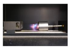
Figure 5.13 Moment of detonation during the positive laser initiation test of complex 12.
