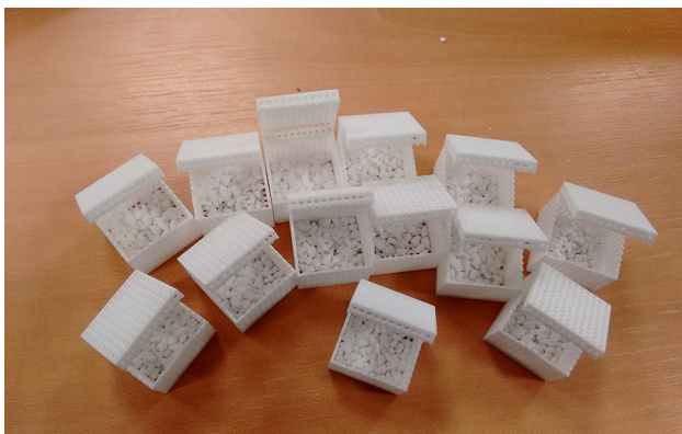
Fig. 2 3D printed grains using box printing method approach
