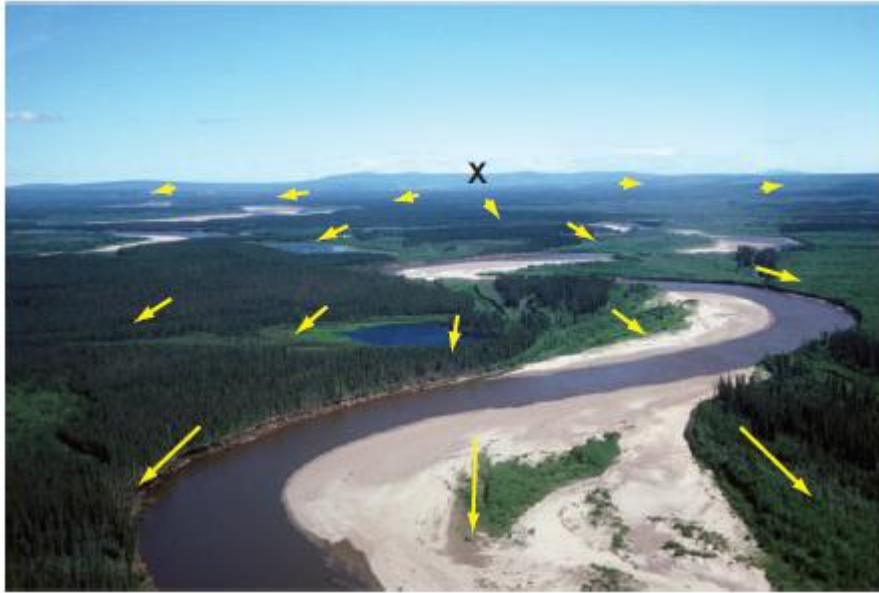
Figure I-2: Optic flow field as created through forward self-motion. The yellow arrows depict the different velocities at different points in the image. These velocity vectors emanate from the black cross. It is the focus-of-expansion and shows, under certain conditions, the self-motion direction. (Britten, 2008)
