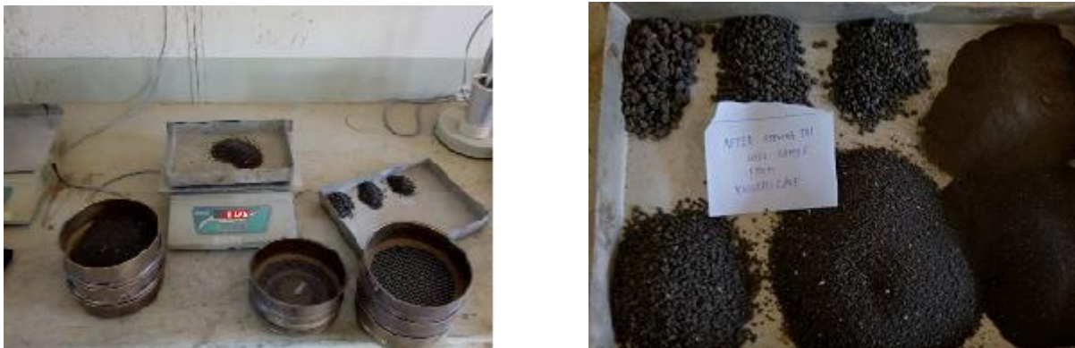
Fig. 4. 5 Field data processing based on the sieve analysis method of Kolleru Lake
