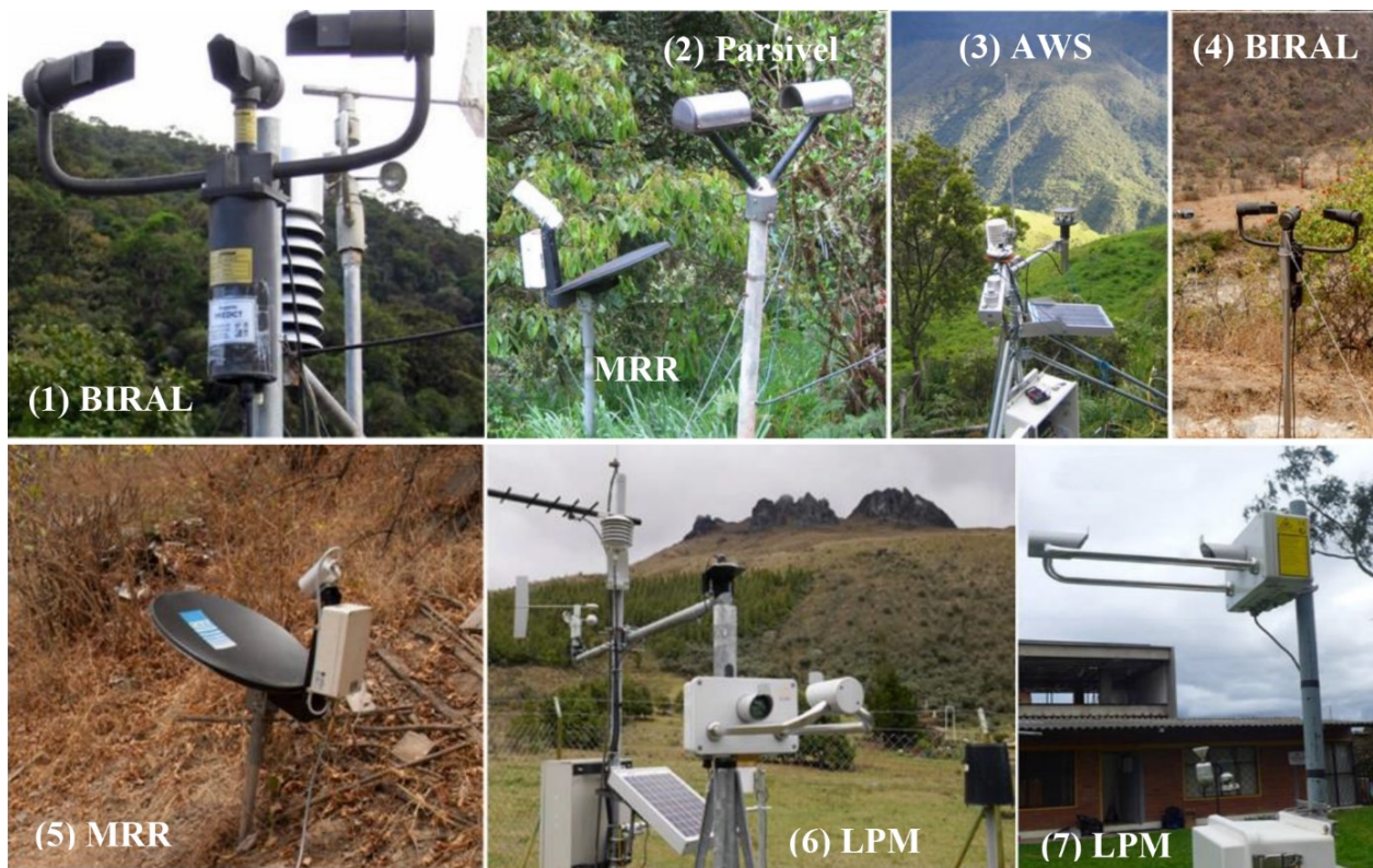
Figure 2.3: Instruments at the disdrometer sites: 1) Biral VPF-730, 2) MRR-2 and OTT Parsivel, and 3) Automatic Weather Station (Campbell) in the ECSF area of the mountain rain forest (for LOXX radar). 4) Biral VPF-730 and 5) MRR-2 at the Laipuna field station in the mountain dry forest (for GUAXX radar). 6) LPM and AWS at La Virgen and 7) LPM at Balzay (for CAXX radar).
