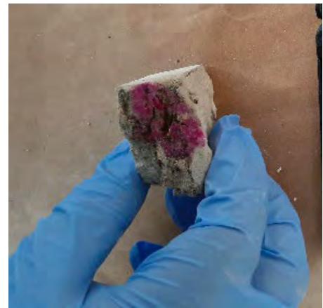
After the application of Phenolphthalein ( C_{20}H_{14}O_4 ) indicator Results: No Carbonation on the Substrate, Partial Carbonation of Stucco
