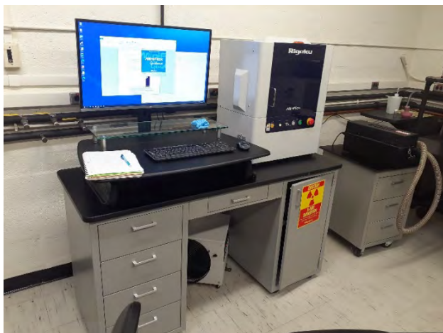
Fig. 5.33 & 5.34 – The computer and the MiniFlex 6G theta-2theta vertical goniometer benchtop powder diffraction system (machine) at the Penn's Laboratory for Research on the Structure of Matter (LRSM). Photos by Author.
