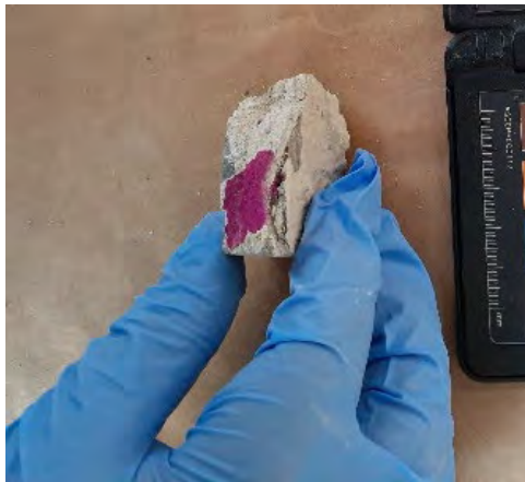
After the application of Phenolphthalein ( C_{20}H_{14}O_4 ) indicator Results: No Carbonation on the Substrate, Partial Carbonation of Stucco
