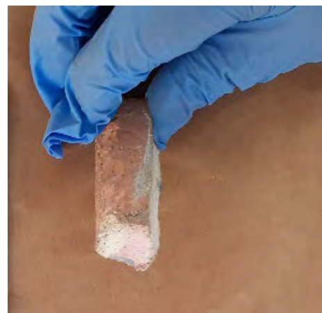
After the application of Phenolphthalein ( C_{20}H_{14}O_4 ) indicator – Results: Clear -Full Carbonation
