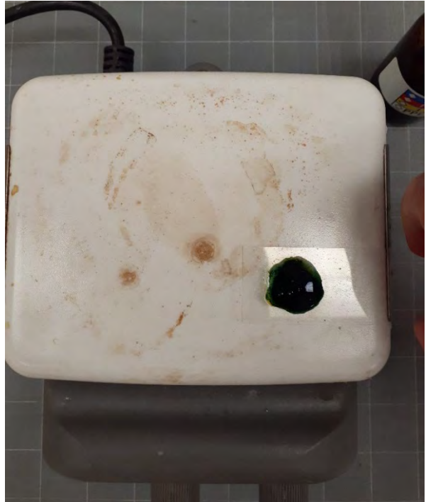
A drop of potassium ferrocyanide soln. was added and it turned to an intense blue (Prussian Blue - C_{18}Fe_7N_{18} )
