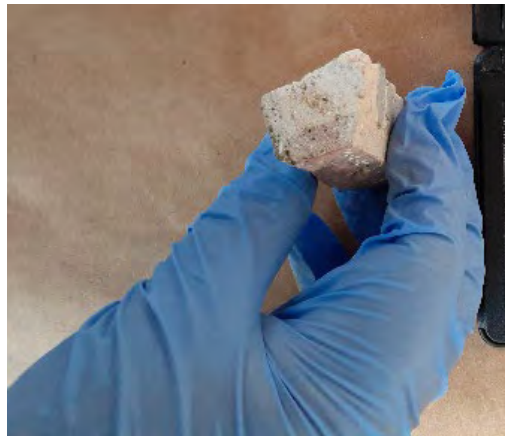
After the application of Phenolphthalein ( C_{20}H_{14}O_4 ) indicator – Results: Clear reaction-Full Carbonation
