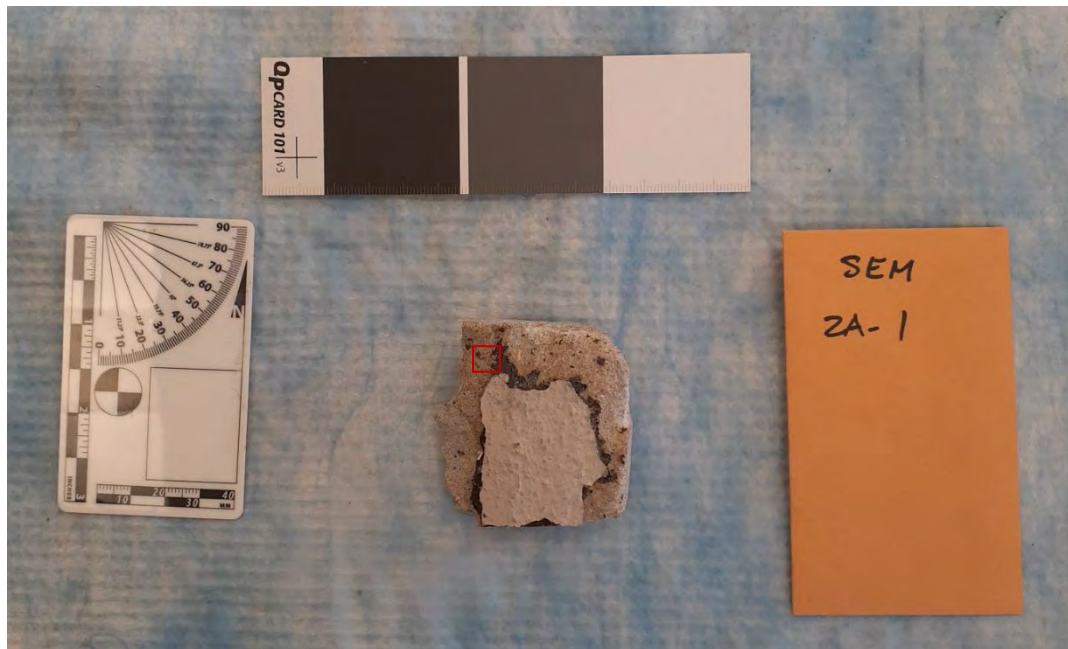
Fig. 5.41 – Sample 2A-1 cross section with selected area before examination on the SEM on August 8 th , 2020. Photo by Author.
