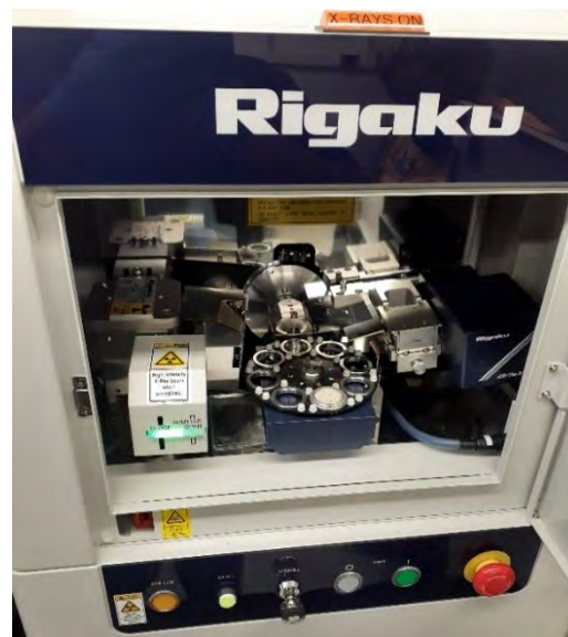
Fig. 5.33 & 5.34 – The computer and the MiniFlex 6G theta-2theta vertical goniometer benchtop powder diffraction system (machine) at the Penn's Laboratory for Research on the Structure of Matter (LRSM). Photos by Author.
