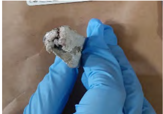
After the application of Phenolphthalein ( C_{20}H_{14}O_4 ) indicator – Results: Clear reaction-Full Carbonation
