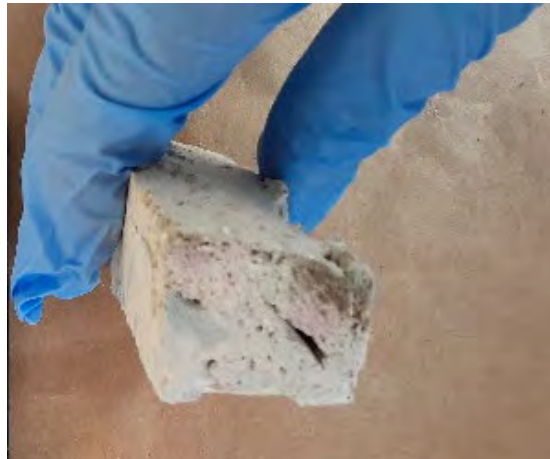
After the application of Phenolphthalein ( C_{20}H_{14}O_4 ) indicator – Results: Clear reaction-Full Carbonation
