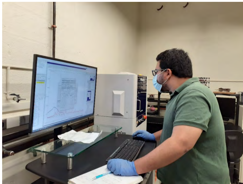
Fig. 5.35, 5.36 & 5.37 – Preparation of Samples for the XRD analysis included passing the powder through a No. 50 Sieve. The results were passed to a data software for interpretation. Photos by Author.
