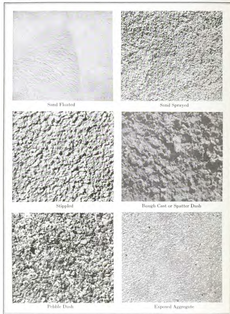
Fig. 3.17 – Standard Stucco Finishes marketed between the 1910s and 1920s. Source: The Stucco House (1921), p. 64.
