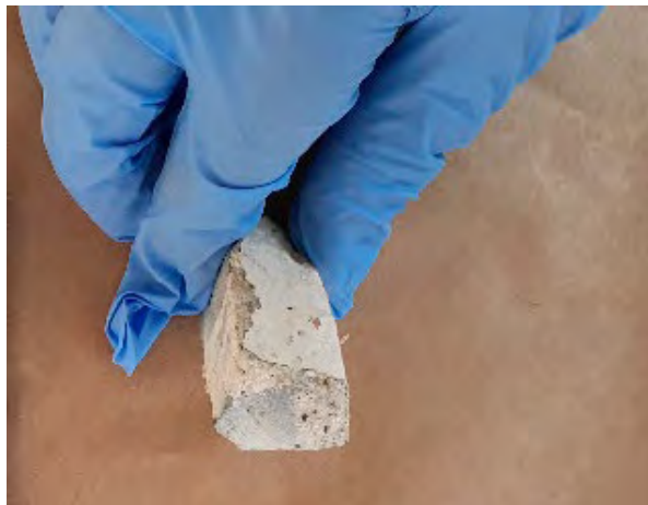
After the application of Phenolphthalein ( C_{20}H_{14}O_4 ) indicator – Results: Clear reaction-Full Carbonation
