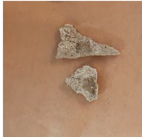
After the application of Phenolphthalein ( C_{20}H_{14}O_4 ) indicator – Results: Clear reaction-Full Carbonation
