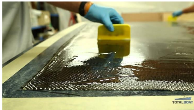
Figure 2-4. Wet layup being performed by hand [6]
