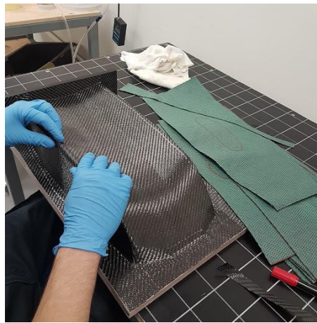
Figure 2-5. Pre-preg being used to create a carbon fiber part [2]
