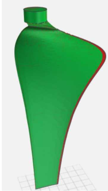
Figure 5-6. Representation of areas too thin for abrasion processes (shown in red)
