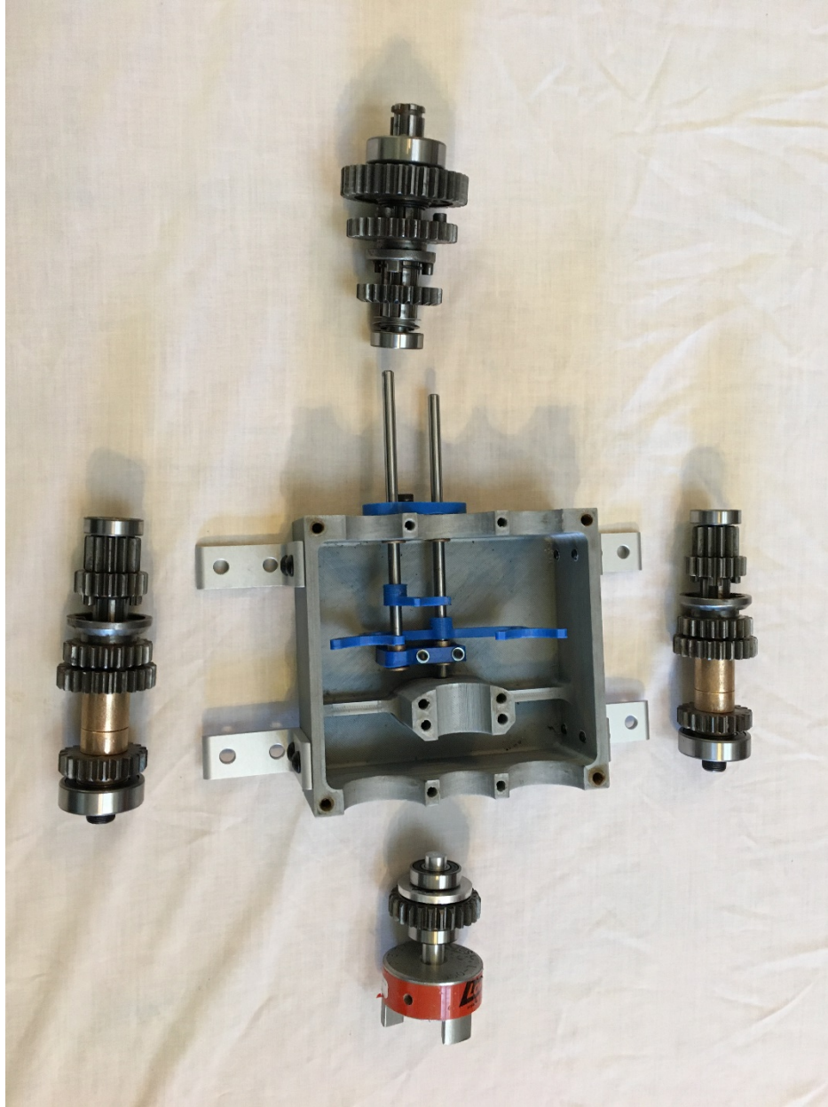
Figure 6.2 3D Printed Mock-Up with Shift Forks
