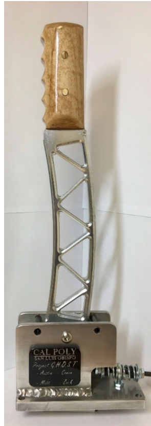
Figure 6.27 Custom Aluminum Shifter for Transmission
