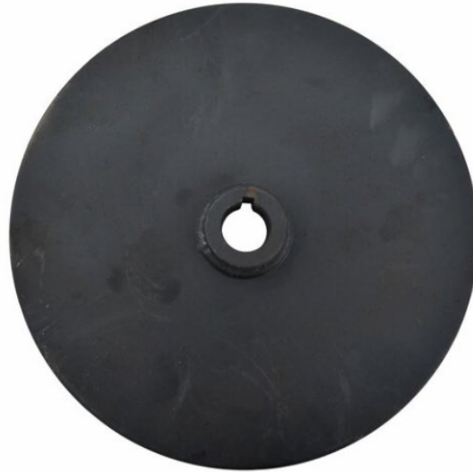
Figure 6.20 Revised Flywheel for the Simulated System Inertia
