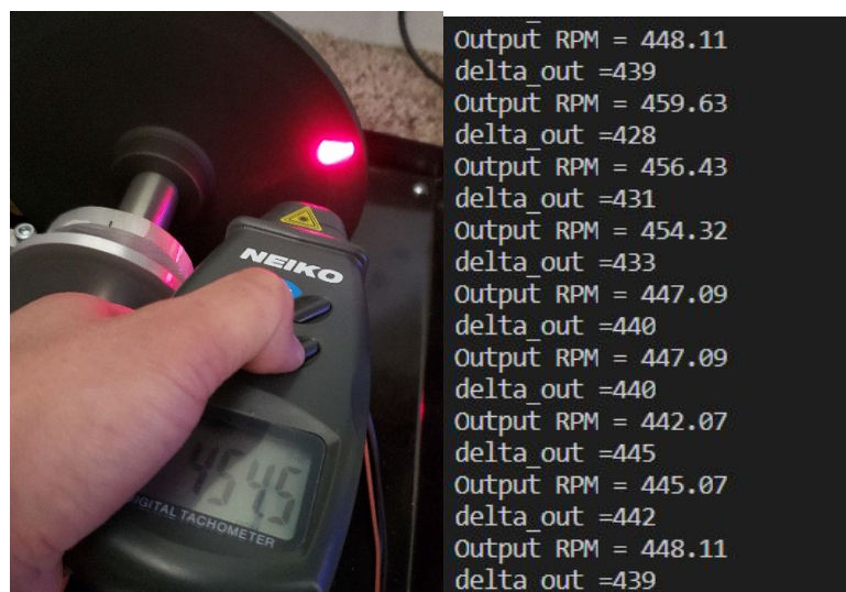
Figure 7.5 RPM Sensor Speed Value and Optical Tachometer Verification
