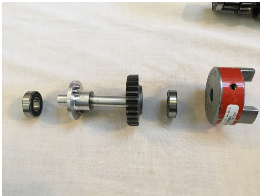
Figure 6.6 Completed Recombining Shaft Assembly
