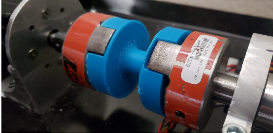
Figure 7.2 Shear Couplers Breaking as Intended and Revised Strengthened Coupler
