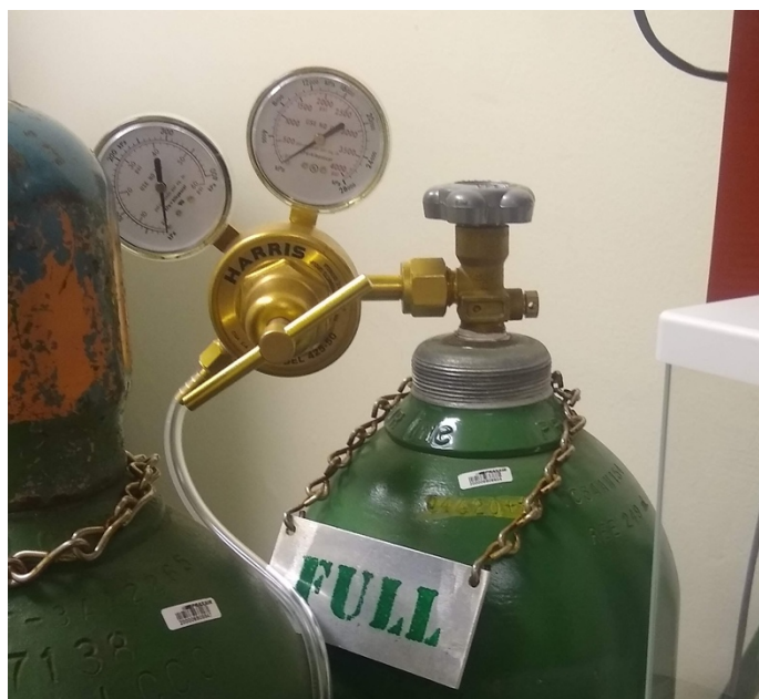
Figure 9: O 2 gas cylinder with the regulator and adapter with tubing attached
