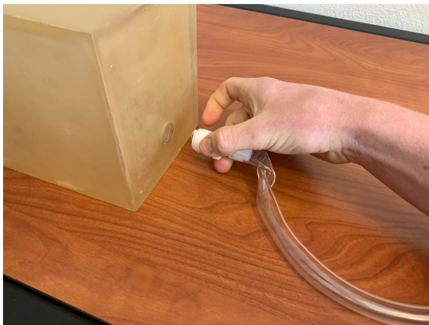
Figure 11: Screwing in the chamber inlet adapter with tubing
