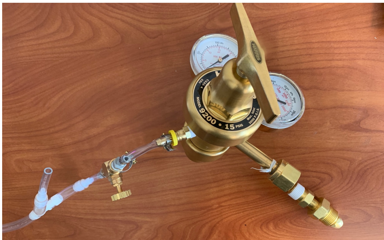
Figure 7: CO2 regulator with adapters, tubing, worm drive clamps, and needle valve
