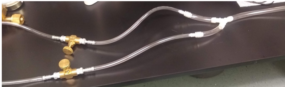
Figure 8: Picture of the brass needle valves with their adapters, tubing, reducers, and wye connector
