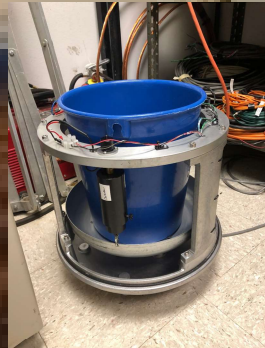
Figure 2. The inside of a Geonor-T200B
