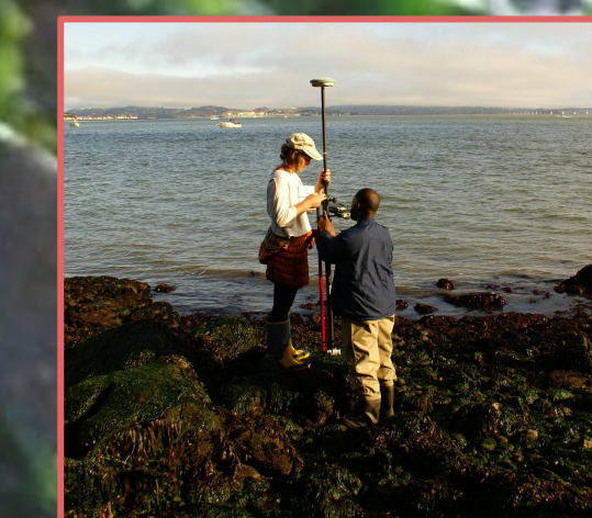
Taking elevation with Real Time Kinematic survey tool, Tiburon, CA. Photo: A. Haigh.
