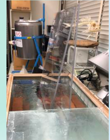
Figure 5. Tank with Plexiglass Guards
