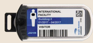
an area dosimeter such as one deployed at SLAC; used to measure an absorbed dose of ionizing radiation
