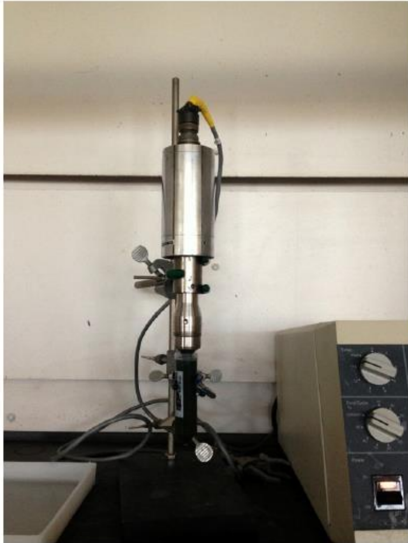
Figure 9- The SHU digester feed was a 10 gVS/L sonicated algal slurry. An analog Branson Sonifier 250 was used to lyse the algal cell walls prior to feeding.
