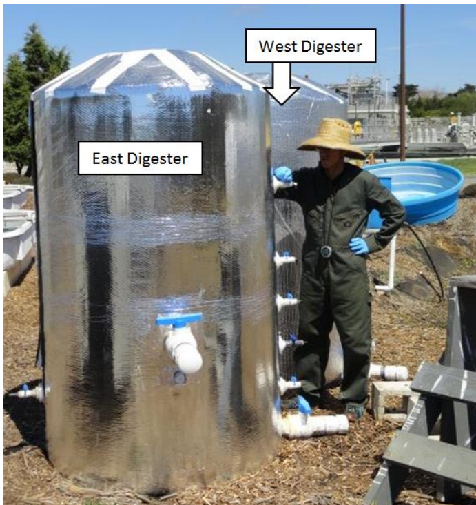
Figure 21- East digester shaded the west digester daily due to proximity of the digesters, located at the AFS.
