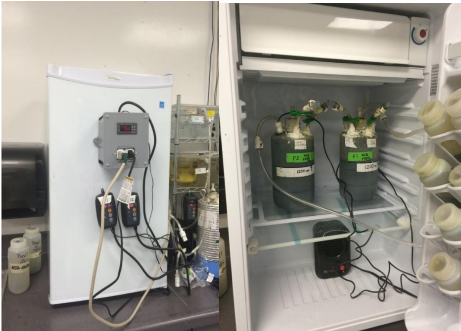
Figure 10 and Figure 11- The temperature-controlled incubator housed the lab-scale digesters for Experiment 3.
