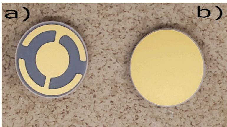
Figure 24. Quartz crystals used in the study a) the bottom side has the electrodes that are in contact with the crystal holder b) the top side where the sample is deposited and is in contact with the CO 2 gas
