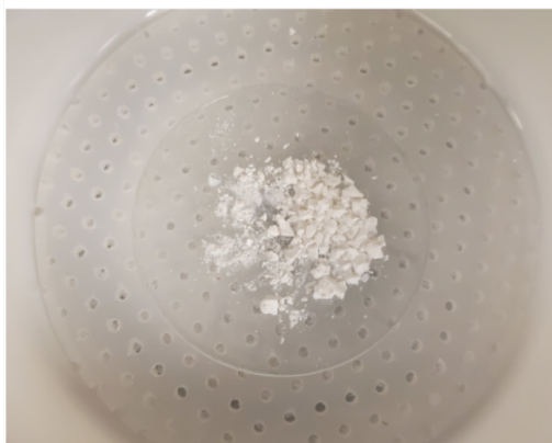
Figure 16. ZIF-8 prepared in methanol a) ZIF-8 solution before drying and centrifugation and b) dry ZIF-8 product
