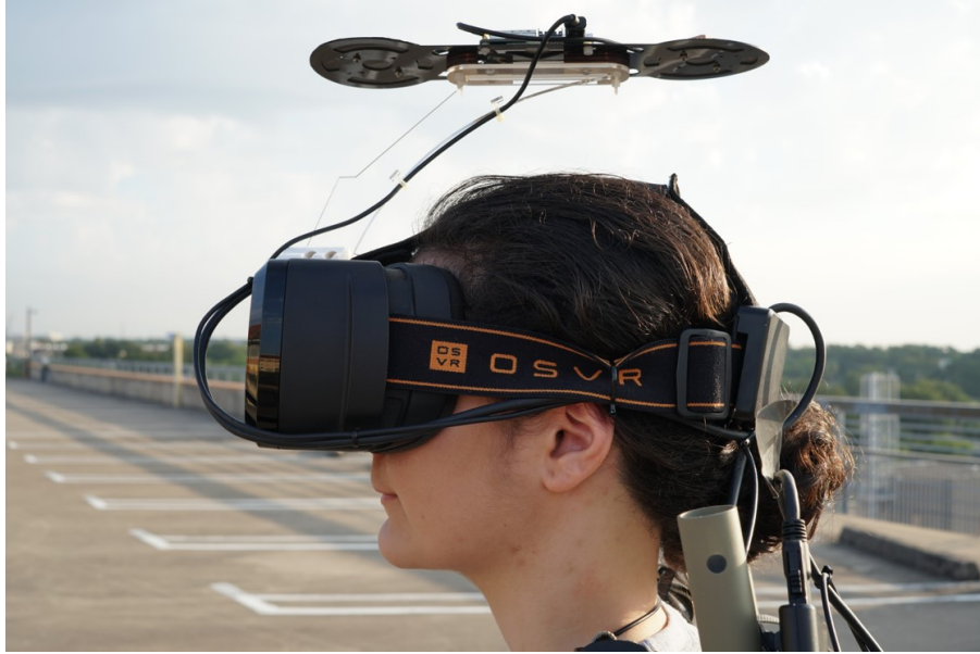
Fig. 1. The Open-World Virtual Reality headset. Measurements from two GNSS antennas and a low-cost inertial measurement unit (IMU) mounted on the plate above the user’s head are combined for centimeter-and-degree-accurate tracking of the VR headset in a global coordinate frame.
